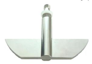
Tolerances Dimensions: Paddle Height 19.0 mm ± 0.5 mm Upper length 74.5 mm ± 0.5 mm Lower length 42.0 mm ± 1.0 mm Size 4.0 mm ± 1.0 mm Radius 1.2 mm ± 0.2 mm Radius 41.5 mm ± 1.0 mm Shaft Diameter 9.4 to 10.1 mm
